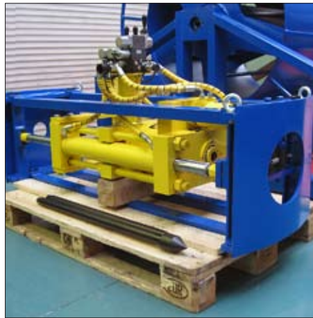
Fig. 1. ACP-20 is a compact solution for pit or well use.
